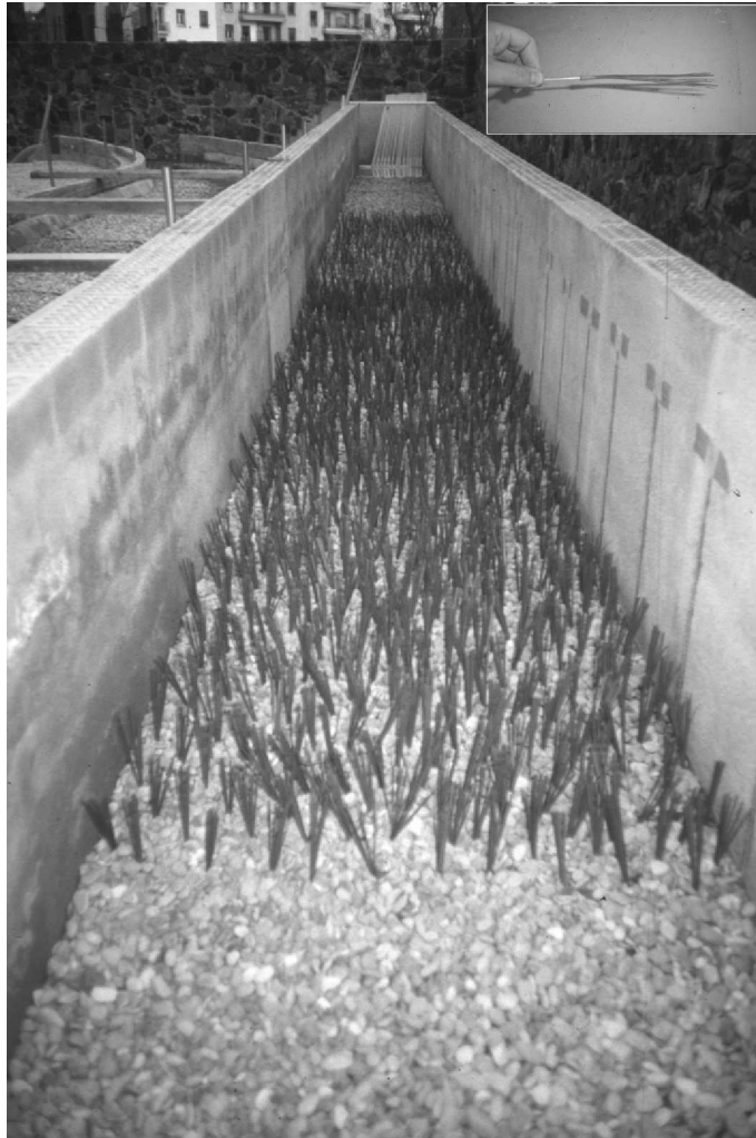
Figure 2.4: Experiments in a 20 m long rectangular flume and detail of the plastic ornamental plant used for the experiments (see incept).
